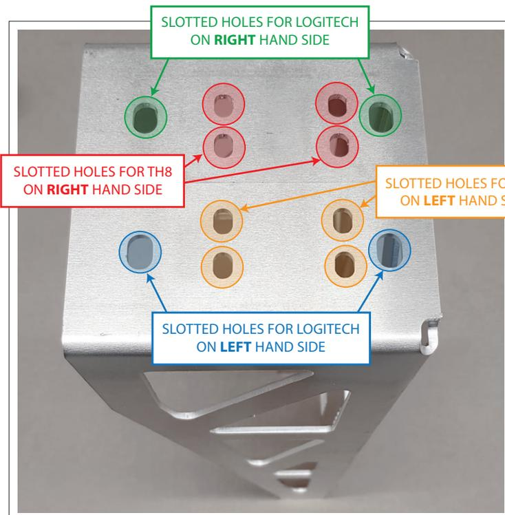
Mount your Logitech shifter to the alloy bracket using two M6x20mm hex bolts, two M6 washers and the slotted holes indicated (blue if using the shifter on the right hand side, or the green holes if using the shifter on the left hand side).
